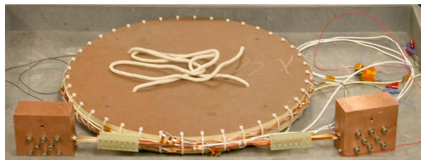
FIGURE 9 One turn coil of 2 m long twisted stacked-tape cable mounted on a side surface of a 0.5 m diameter disk.
