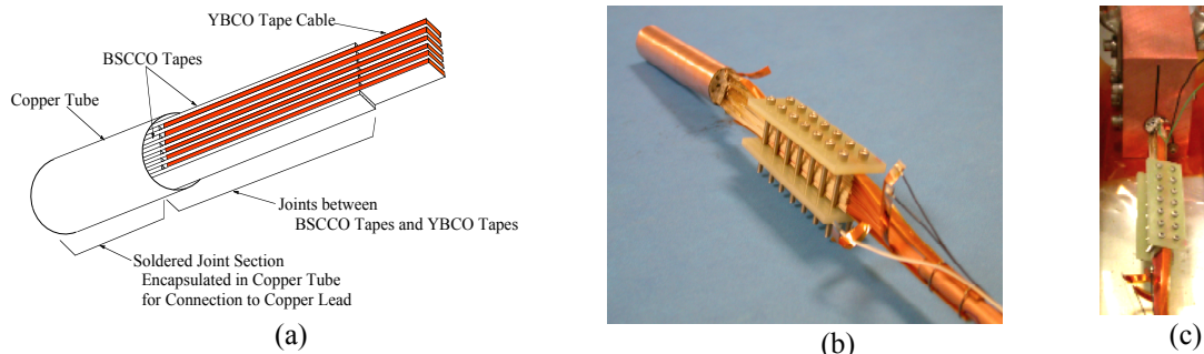
FIGURE 2 Copper-BSCCO-YBCO termination. (a) Schematic illustration of YBCO tape sandwiched between BSCCO tapes. (b) Fabricated 44-BSCCO-tape terminator (left) for a 43 stacked-tape YBCO conductor (right). Stacked YBCO tapes were sandwiched between the BSCCO tapes (center) which were clamped with 70 mm length G10 plate without soldering. The BSCCO tapes were soldered in a copper tube (left). (c) The copper tube was clamped on a copper block to connect to a copper power cable.
