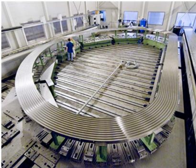
Fig. 3. The EU SIMIC regular radial plate prototype after machining completion.
