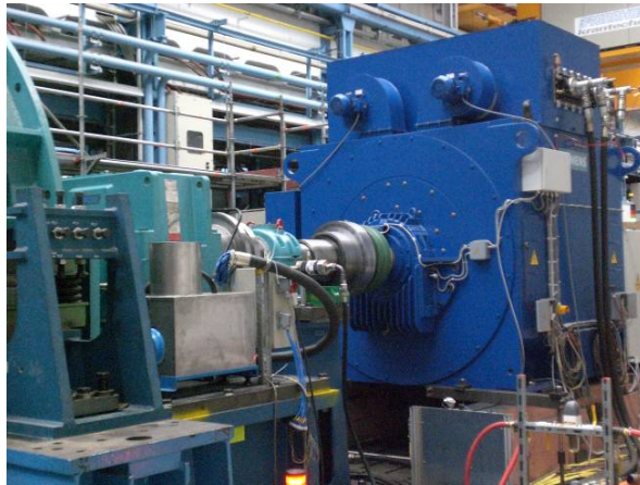
Fig. 4. The HTS-3 motor on test bed coupled to the load machine.
