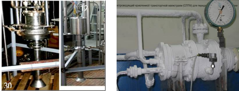
Fig.12. Cryogenic pumps with HTS motor. Left – 30 kW and 12KW pumps, right – the HTS motor during preliminary tests.
