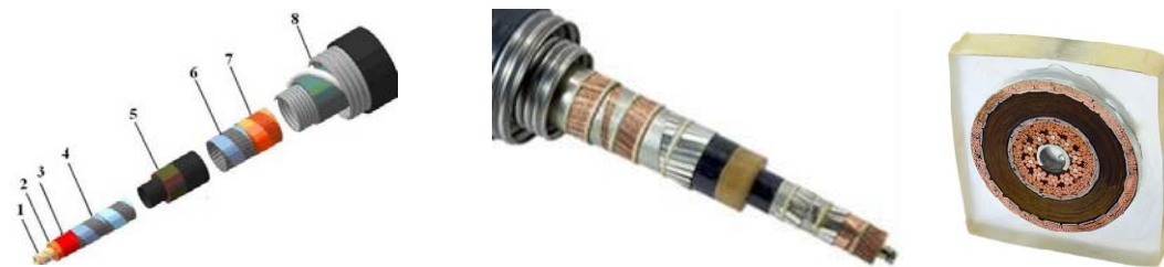
Fig.1. Artis’s conception (right) , photo of the cable model (center) and cross-section of one phase of the 200 m cable (right). 1-Former- a spiral of stainless steel, surrounded by a bundle of wires made of copper and stainless steel, wrapped in copper tape - 2 and 3; 4 - Two layers of HTS tapes; 5 - high-voltage paper insulation; 6 - HTS shield -7- flexible copper strips to protect shield, wrapped by tapes of stainless steel; 8- flexible cryostat, 200 m long.
