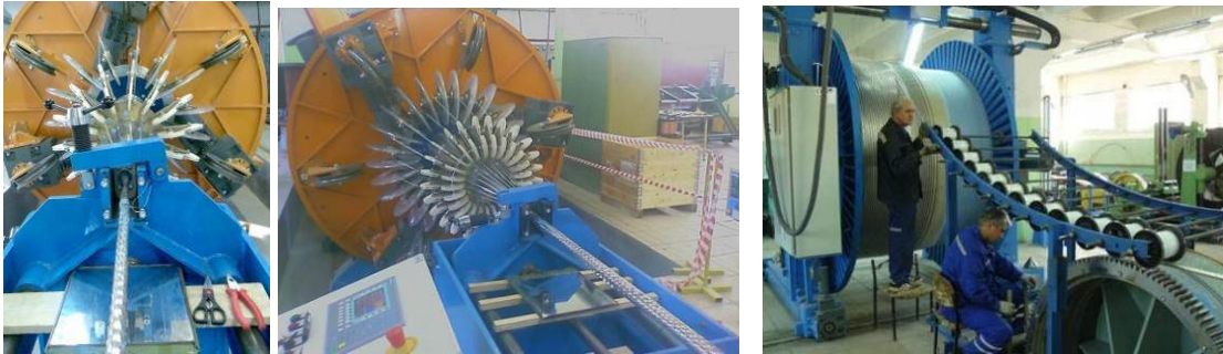
Fig. 2. Production of the 200 m HTS cable. From left to right: layer's twisting, superconducting shield's twisting, cable on a take-on drum.
