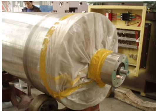
Fig. 4 Total leak rate detection
