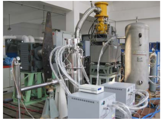
Fig. 10 Cryogenic cooling system test.
