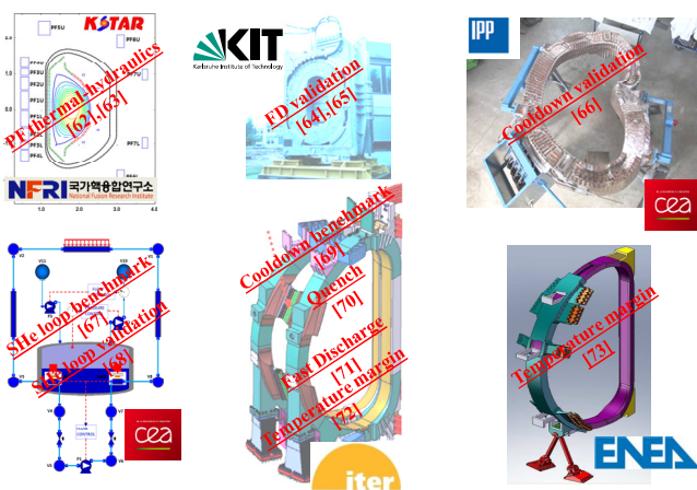
Figure 2. Benchmarking, validation and applications of the 4C code so far, highlighting for each experiment the issues addressed and the major laboratories with which these exercises were carried out. Clockwise from bottom left: CEA Grenoble supercritical helium loop HELIOS [58]; KSTAR SC magnet system [59]; the TFMC monument at KIT; one non-planar coil of the W7-X stellarator [60]; one TF coil of the JT60-SA tokamak [61]; a pair of ITER TF coils.
