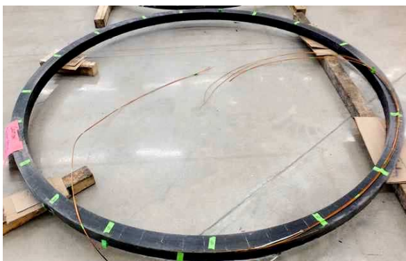
Fig. 5. A single cyclotron gas-stopper magnet coil that has an average diameter of 2470 mm and a cross-section of 80 by 80 mm.
