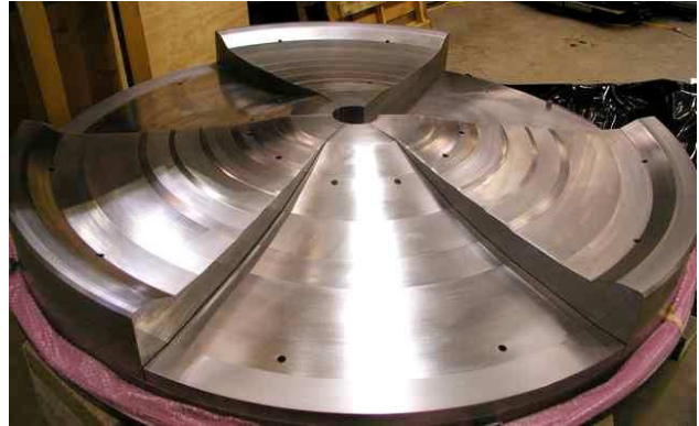
Fig. 6. The machined pole-piece sectors for the magnet. The outside diameter of the pole is 2200 mm.
