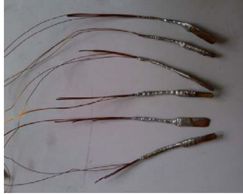
Fig. 2 (b). NbTi joint samples, (a) before press operation, after press operation.
