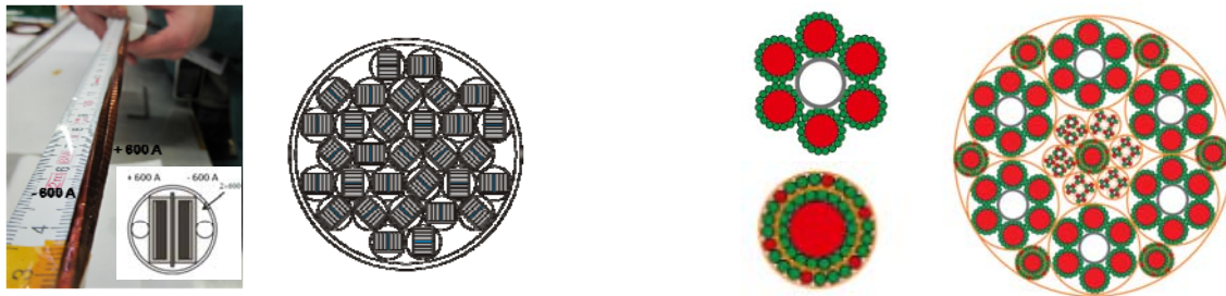
Fig. 2. Left: \text{MgB}_2 Twisted-pair cable, \Phi=5.6 mm and Twisted-Pair assembly of 2 \times 25 \times 600 A cables for LHC P7, \Phi=40 mm. Right: 20 kA \text{MgB}_2 cable, \Phi=6.5 mm (top), 2 \times 3 kA \text{MgB}_2 concentric cables, \Phi=8.2 mm (bottom), 150 kA cable assembly for LHC P1 and P5 ( 6 \times 20 kA, 2 \times 7 \times 3 kA, 4 \times 0.4 kA, 18 \times 0.12 kA), \Phi=65 mm
