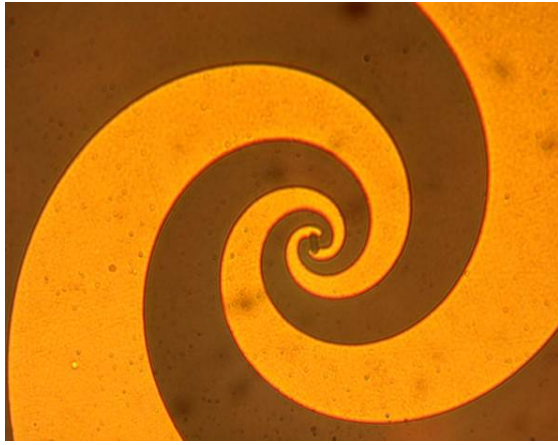
Fig. 1. Optical image of spiral antenna device #1 with bridge dimensions of 6\ \mu\text{m} (L) \times 4\ \mu\text{m} (W) \times 15\ \text{nm} (T).
