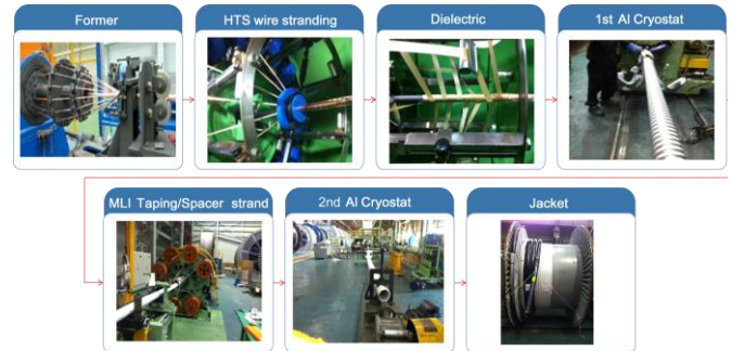
Fig. 2. Fabrication of HTS DC cable by manufacturer LSC
