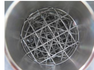
Fig. 4. Magnetic filter of separation unit. (Inlet side in filter condition B)
