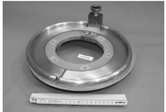
Fig. 2. Double-pancake test coil #2. The windings are below the copper sheet and copper tube, which is part of a heat pipe system for liquid Ne to cool the coil to 30K. The ruler below is marked in cm.
