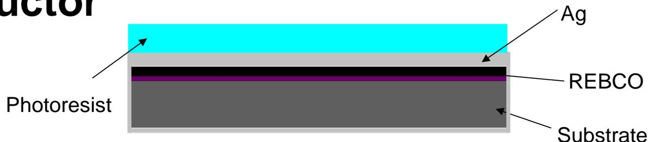
2. Transfer pattern from mask to photoresist
