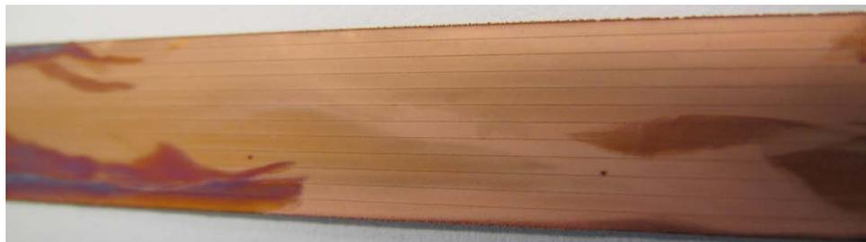
12-filament wire with 10  $\mu\text{m}$  thick fully striated copper stabilizer using benign copper chemistry
