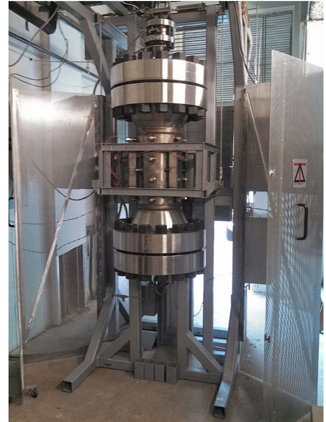
100 bar, 900 °C Deltech furnace with 14 cm diam. X 50 cm long hot zone
