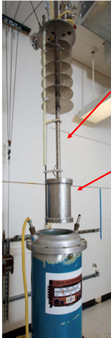
Superconducting shield 2mm thick Nb
