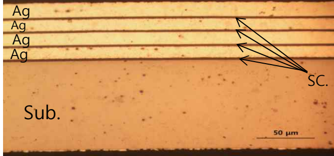
Longitudinal cross-section of 4-Superconducting layered HTS wire
