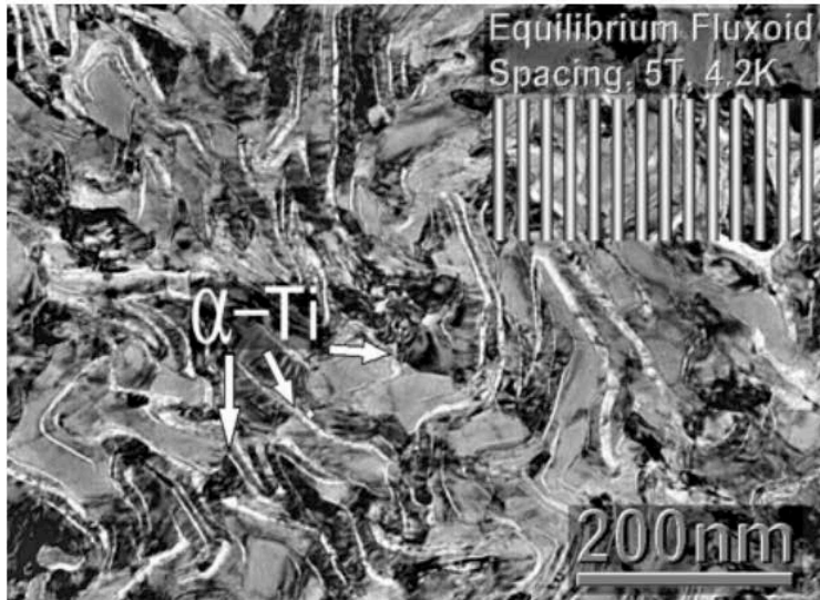
\alpha -Ti ribbons in a Nb-Ti alloy (D. Larbalestier & P. Lee)
