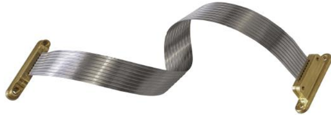
Fig. 1. Eight-trace Maybell cable prototype manufactured using linearly actuated mechanical stage with laser welding. Two sheets of 1 mil thick NbTi foil are welded around PFA-coated NbTi wires with a continuous laser weld.
