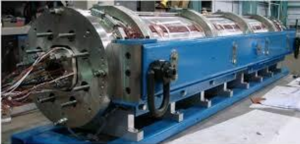
3.4 m long Nb 3 Sn magnet [G. Ambrosio, et al. IEEE TAS 17 (2007) 1035]
