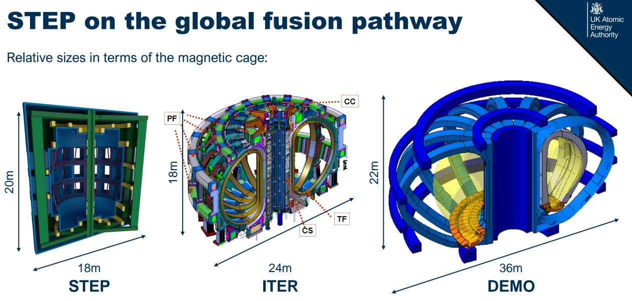
The functionality of DEMO at a size less than ITER thanks to HTS (and the spherical tokamak).
