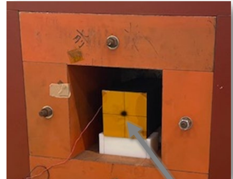
Beam mark produced by the extracted beam
