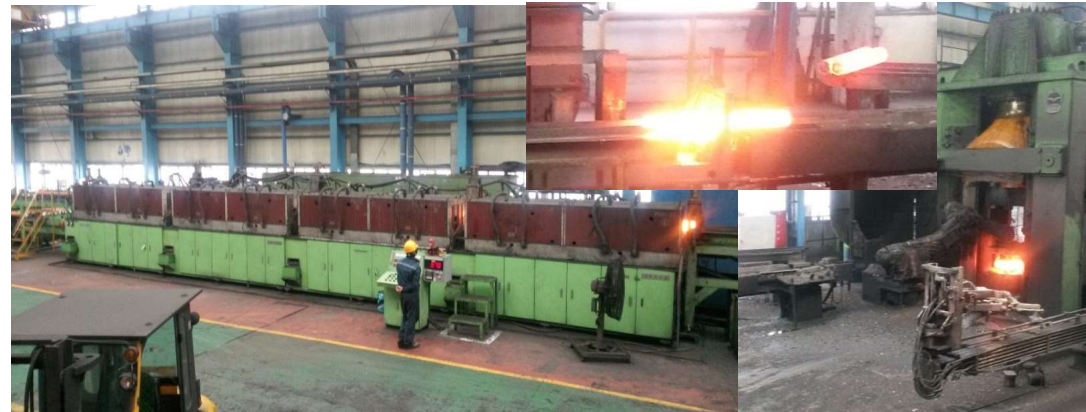
▲ Forging company with iron metals using Gas furnace and electric furnace
