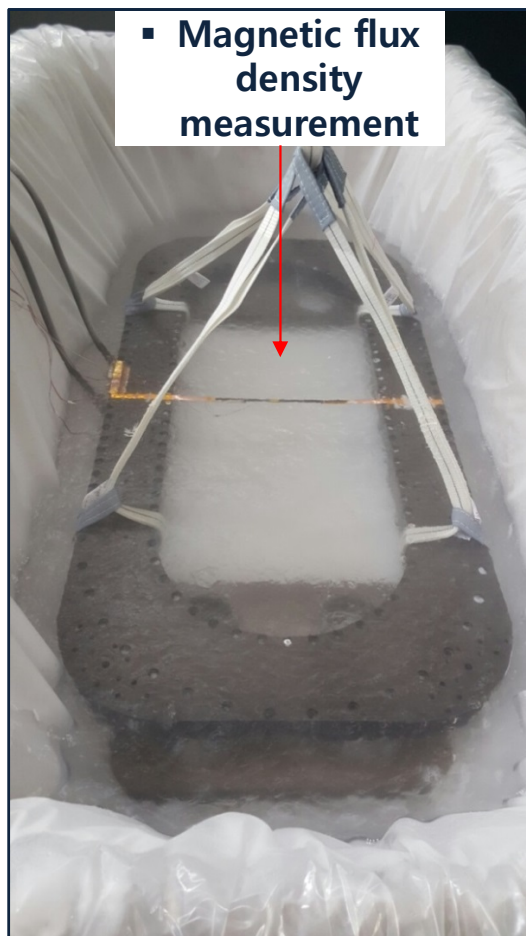
▲ Cooling HTS magnet in liquid nitrogen, 77.4 K
