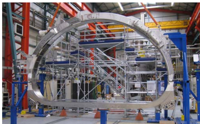
Fig. 5: TF coil pre-assembly with Outer Intercoil Structure
