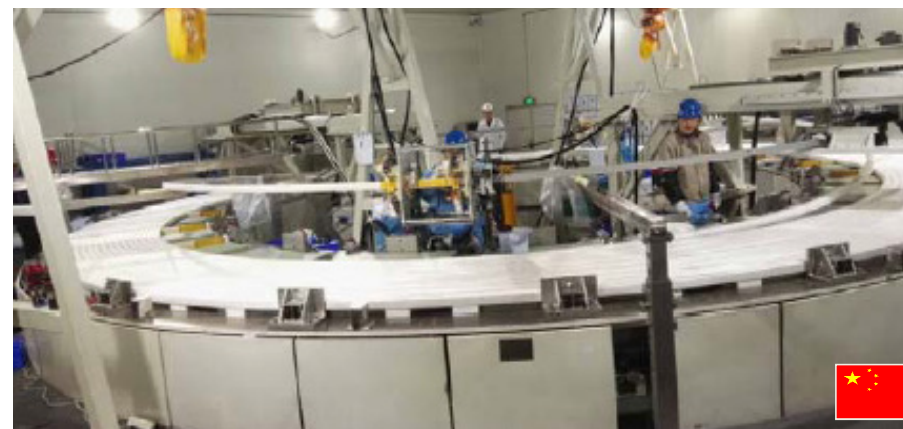
2nd PF6 DP Winding (underway) 8 th DP now complete
