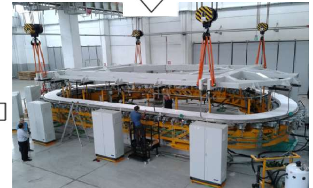
DP Loading into Vacuum Impregnation Mold (radiation-hard cyanate ester resin)
