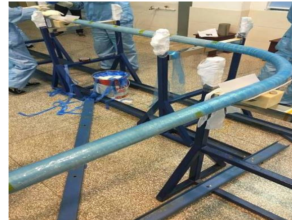
Silicon wrap to compress during curing
