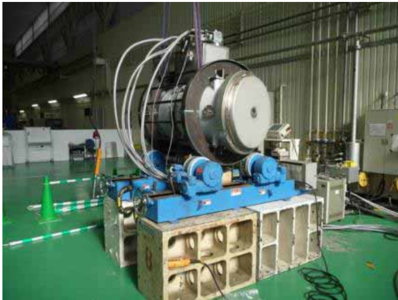
photographs of rotating test (prototype magnet)
