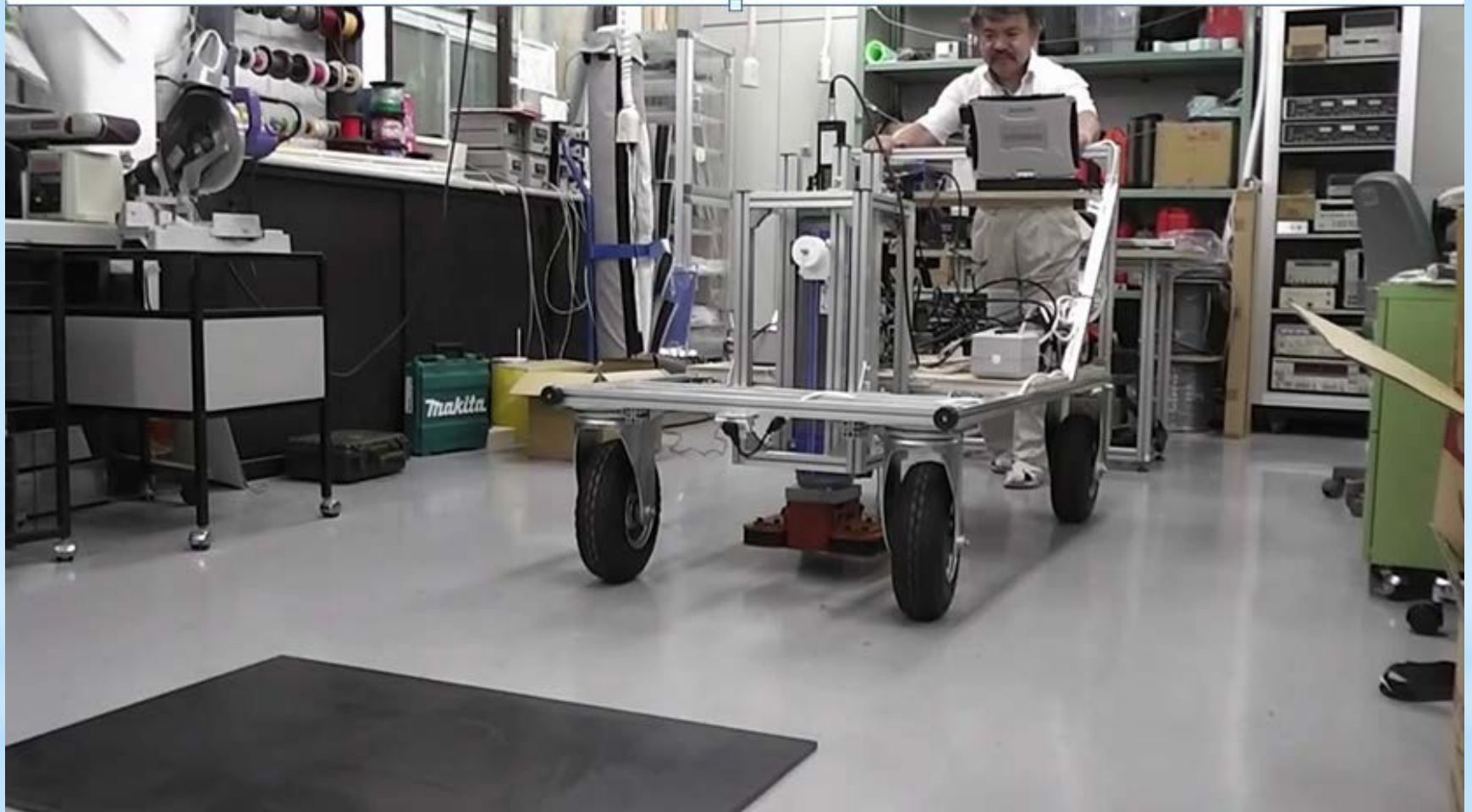
NDE system using a cart for field test
