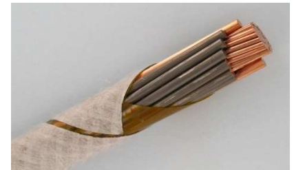
Reacted wires with mechanical properties suitable for cabling operation using industrial machine
