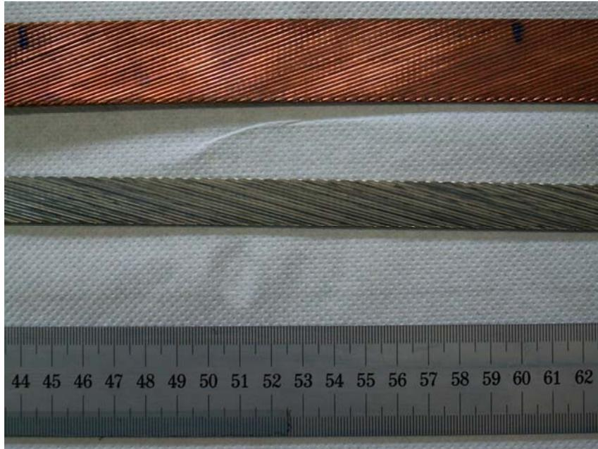
**Fig.3.** Photo of a 40-strand Rutherford-type cable produced by LBNL with SMI/NED wire (top) compared to a 28-strand LHC inner layer cable (bottom).
