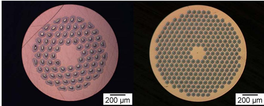
**Fig.1.** Cross-sectional views of wires developed within the framework of the CARE/NED activity: (a) Internal Tin wire produced by Alstom/MSA (left) and (b) Powder-In-Tube wire developed by SMI (right).
