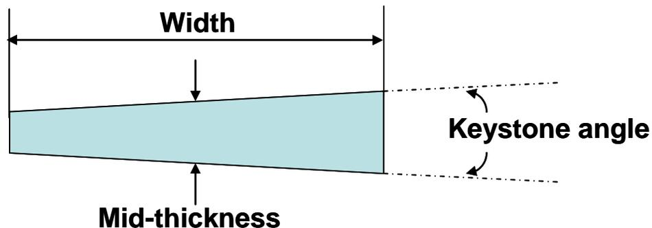
**Fig.4.** Schematic cross section of a Rutherford-type cable, defining the main dimensional cable parameters mentioned in Table 2.
