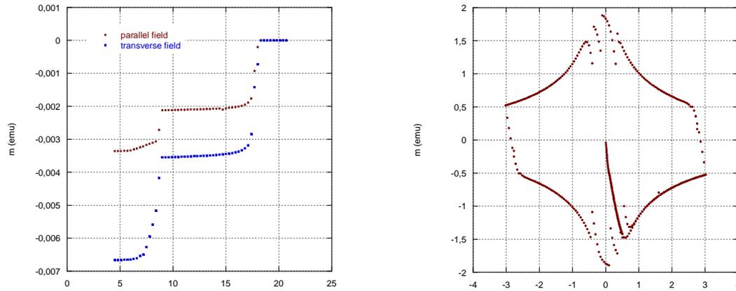
**Fig.2.** Magnetization measurements on SMI/NED wire: (a) as a function of temperature (left) and (b) as a function of field (right; courtesy of P. Fabricatore and M. Greco, INFN-Genoa, C. Ferdeghini, INFN-Genoa and U. Gambardella, INFN-Frascati).
