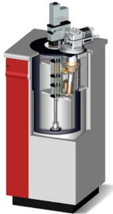
**Fig. 5.** The MPMS EverCool dewar and cabinet assembly. The 1<sup>st</sup> stage of the cryocooler is attached to the thermal shields in the dewar, while the second stage recondenses the helium gas that would otherwise be lost.
