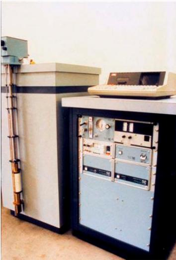
**Fig. 2.** The Mark I – the first Quantum Design MPMS. This 2-Tesla MPMS used an SHE Model 30 SQUID controller and the user interface was written in BASIC on a Hewlett-Packard HP-85 computer. The system was shipped to Prof. Robert Shelton at Iowa State University in July 1984.
