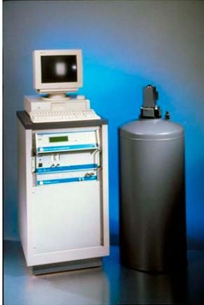
**Fig. 3.** An early PPMS system. This instrument is shown with the sample drive mechanism (on the top of the dewar and probe assembly) that provides the sample motion for the PPMS AC-DC Magnetization (ACMS) measurement option.
