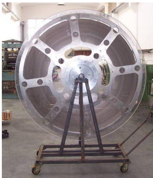
Fig. 3. 1.6 Km of stabilized multifilamentary MgB_2 tape fabricated in our laboratory by the powder in tube method; now this technology is used by Columbus Superconductors.
