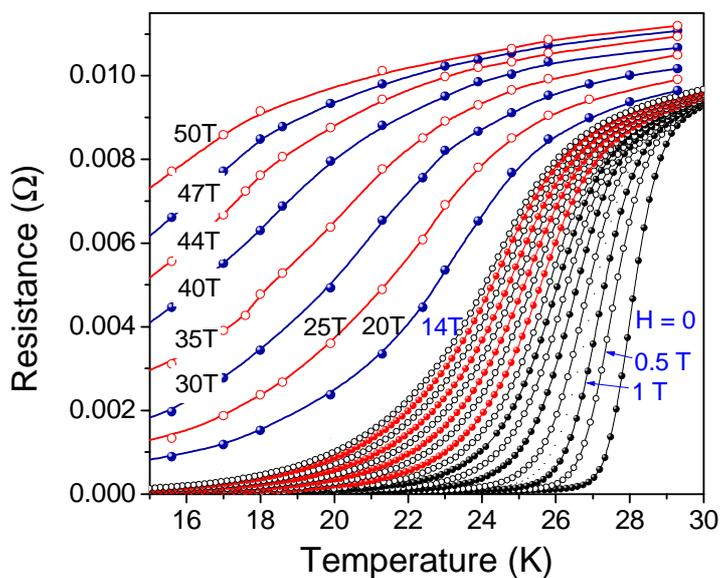
**Figure 1.** Temperature dependence of the resistance of an AD sample from both DC and pulsed field measurements.
