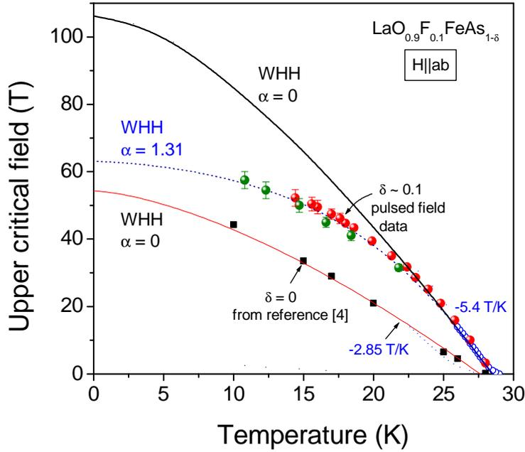
**Figure 2.** Temperature dependence of  $B_{c2}^{ab}$  for  $\text{LaO}_{0.9}\text{F}_{0.1}\text{FeAs}_{1-\delta}$ . Data for the AD sample from DC ( $\circ$ ) and pulsed field measurements ( $\bullet$  - IFW Dresden,  $\bullet$  - FZD) in comparison with data ( $\blacksquare$ ) for a clean reference sample [4]. Solid lines: WHH model without PLB. Dotted line:  $B_{c2}^p(T)$  for  $\alpha = 1.31$  (see text).
