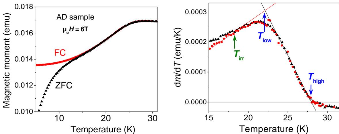
**Figure 4.** Temperature dependence of the magnetic moment  $m(T)$  (left) and of  $dm/dT$  (right) for the AD sample measured at 6T applied after zero-field cooling (ZFC) and before cooling (FC).
