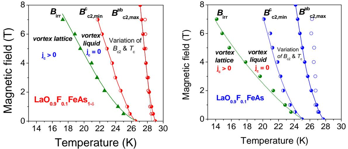
**Figure 5.** Temperature dependence of the highest and the lowest upper critical field  $B_{c2,max}^{ab}$  and  $B_{c2,min}^c$ , respectively, and of the irreversibility field  $B_{irr}$  for the AD sample (left) and the clean reference sample (right). In the case of  $B_{c2,max}^{ab}$ , data from magnetization (open circles) and from resistance measurements (filled circles) are compared.
