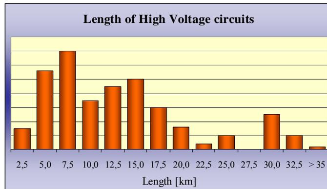
**Figure 3.** Length of HV circuits in Allianter's grids
