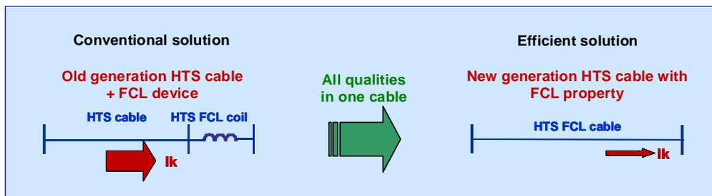
**Figure 2.** Schematic showing the advantages of HTS cable with integrated FCL property
