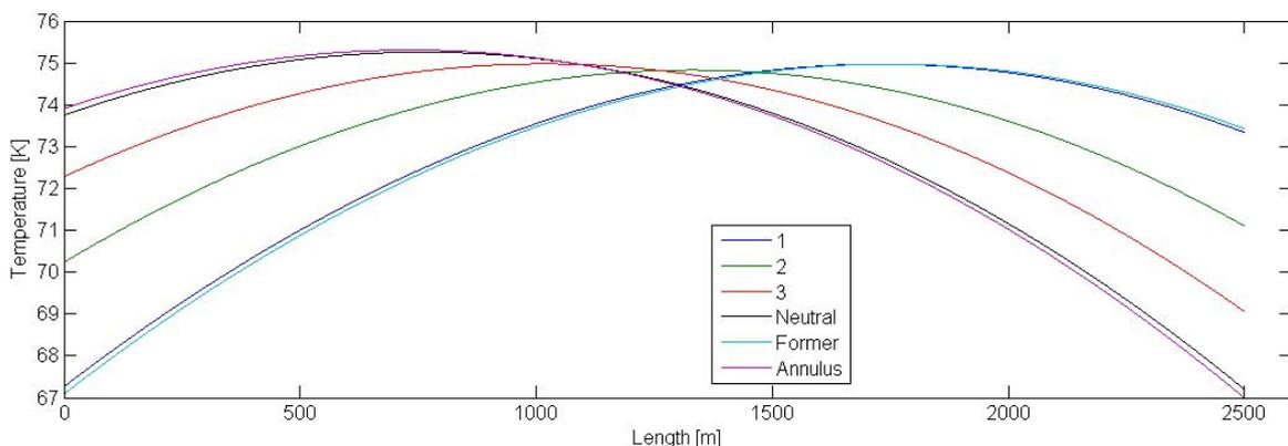
**Figure 4.** Simulated temperature profile of a 2.5 km long 50 kV HTS Triax® FCL cable using the present-status performance values for the AC and cryostat losses. The modeled system has one cooling station at each end
