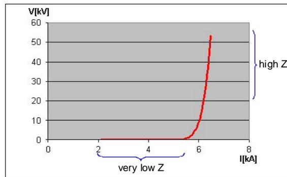
**Figure 1.** A schematic of the non-linear voltage vs. current characteristics of HTS cables
