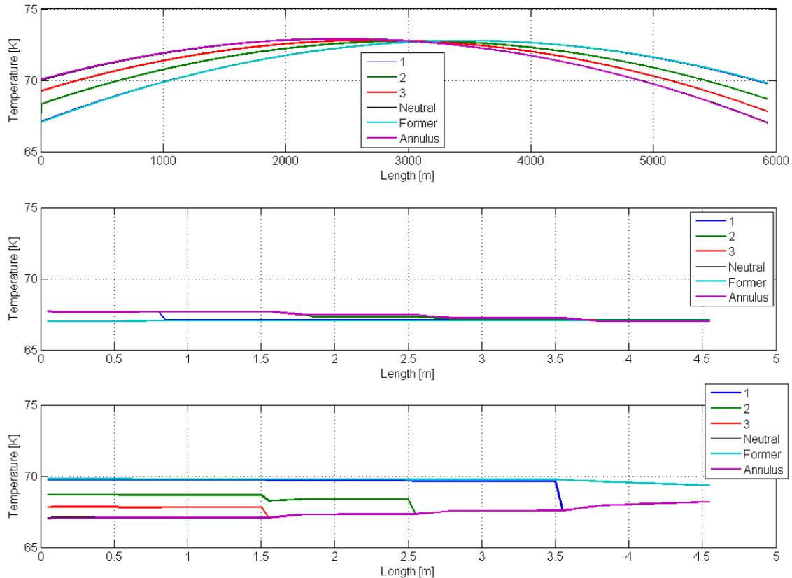
**Figure 6.** Thermal profile of a 6 km long 50 kV HTS Triax® FCL cable using the target performance parameters shown in table 1. The temperature profiles inside the terminations are shown separately with a different length scale.
