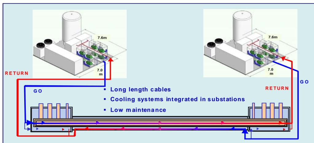
**Figure 5.** Cooling system
