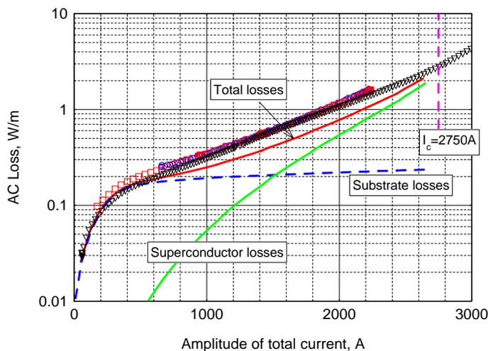
**Figure 6.** AC loss evaluation data, log Y scale at different runs. At dashed vertical line, peak current reaches  $I_c$ . Symbols – experimental data, solid lines – calculations.
