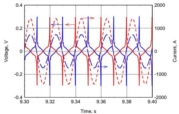
**Figure 5.** Typical current and voltage signals during measurements in AC mode. Voltage of inner layer is reversed to be seen well. Higher current is the total cable current, lower current is the current in the inner layer.
