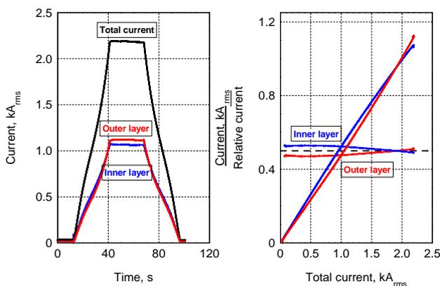
**Figure 4.** Example of AC current run to 2.2 kA<sub>rms</sub> (left) and current distribution among layers (right). Right: rising curves – total layer current; flatter curves – fractional current.
