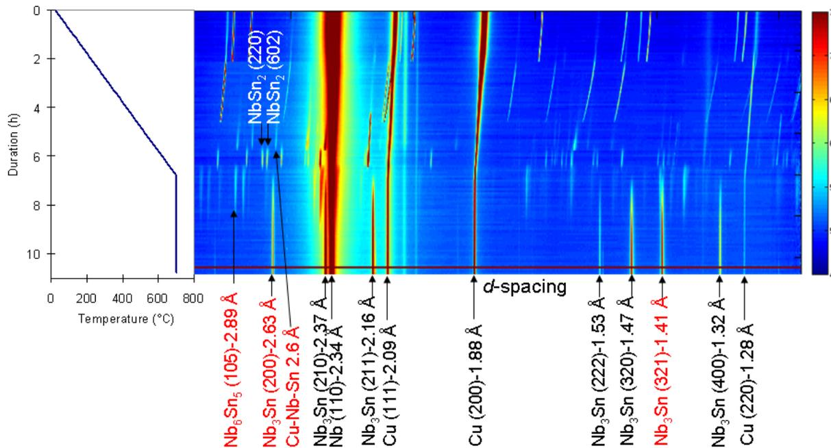
Figure 3: Colour intensity plot summarising 130 diffractograms that have been acquired during *in-situ* HT of the Tube Type  $\text{Nb}_3\text{Sn}$  strand with a ramp rate of  $100\text{ }^\circ\text{C/h}$  and an additional  $4\text{ h-}700\text{ }^\circ\text{C}$  isothermal step. The reflections that were used for peak area measurements are labeled in red and white. The  $d$ -spacing axis is inverted with respect to figure 2.
