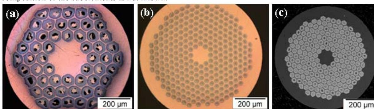
Figure 1: Cross sections of the three strand samples investigated, (RRP billet #7419 with 54 subelements,  $\varnothing=0.80$  mm, non-Cu=51.9 vol.% (a), PIT B215, with 288 subelements,  $\varnothing=0.80$  mm, non-Cu=45.1 vol.% (b), and Tube Type T1505 with 192 subelements,  $\varnothing=0.70$  mm, non-Cu=46.5 vol.% (c)).
