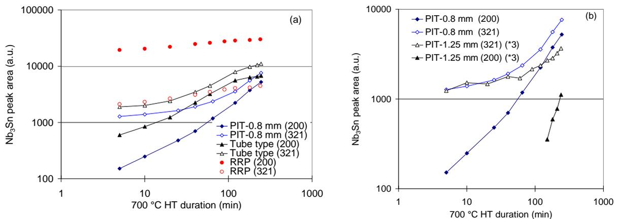
Figure 6: Comparison of  $Nb_3Sn$  (200) and (321) peak area evolution vs. 700 °C HT duration for the 3 different strand types (a) and for PIT-1.25 and PIT-0.80 (b). The peak areas of the PIT-1.25 mm strand have been multiplied by a factor of 3.
