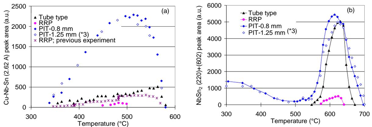
Figure 4: Cu-Nb-Sn ( $d$ -spacing=2.62 Å) (a) and  $\text{NbSn}_2$  (220)+(602) peak area (b) evolution in the different strand samples during a 100 °C/h HT. The peak areas of the PIT-1.25 mm strand have been multiplied by a factor of 3.
