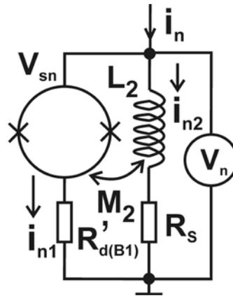
**Fig. 2.** The noise equivalent circuit of SBC. The noise current  $i_n$  flows from the output of the preamplifier into the two parallel branches  $B_1$  and  $B_2$  and generates the noise voltage  $V_n$  across each branch.
