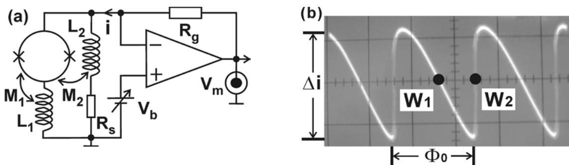
**Fig. 1.** (a) Voltage biased SBC circuit with preamplifier. (b) SBC  $I-\Phi$  characteristic of  $B_1$ , measured at  $V_m$  under the critical condition of  $M_1 \cdot (\partial i/\partial \Phi) = 1$ . The maximum current modulation amplitude ( $\Delta i$ ) of SQUID sample #1 with inductance  $L_s \approx 300$  pH was approximately  $3\mu\text{A}$ .
