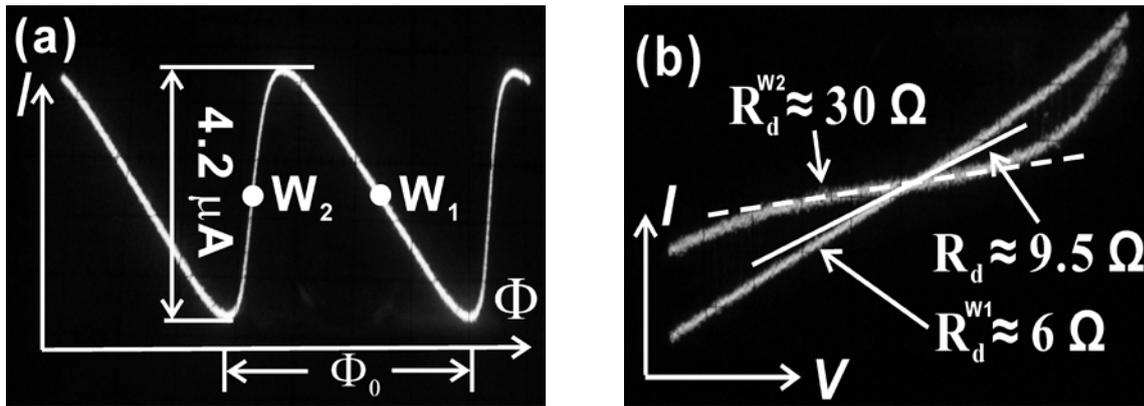
**Fig. 3.** Measured  $I-\Phi$  (a) and  $I-V$  (b) characteristics of SBC (SQUID sample #2). The two curves (near the working point) in (b) cross at the two working points  $W_1$  and  $W_2$ . The  $I-V$  curve of the magnetometer without SBC is indicated by the white continuous line.
