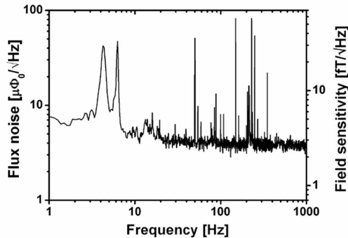
**Fig. 4.** The measured flux noise spectrum and its corresponding field sensitivity of a helium cooled SQUID magnetometer with a SQUID inductance of 350 pH.
