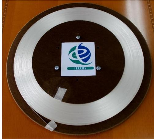
FIG. 1 The world's first 100 meter-class iron-based superconducting wire developed in the Institute of Electrical Engineering, Chinese Academy of Sciences (IEECAS).
