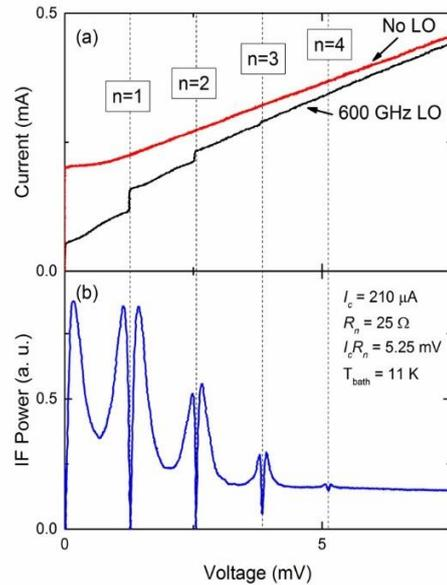
**Fig. 1.** (a) Current vs voltage for the junction under 600 GHz irradiation (black) and without pumping (red). (b) IF power in the same junction been irradiated at 600 GHz showing the local minima occurring at the voltage corresponding to the Shapiro steps.
