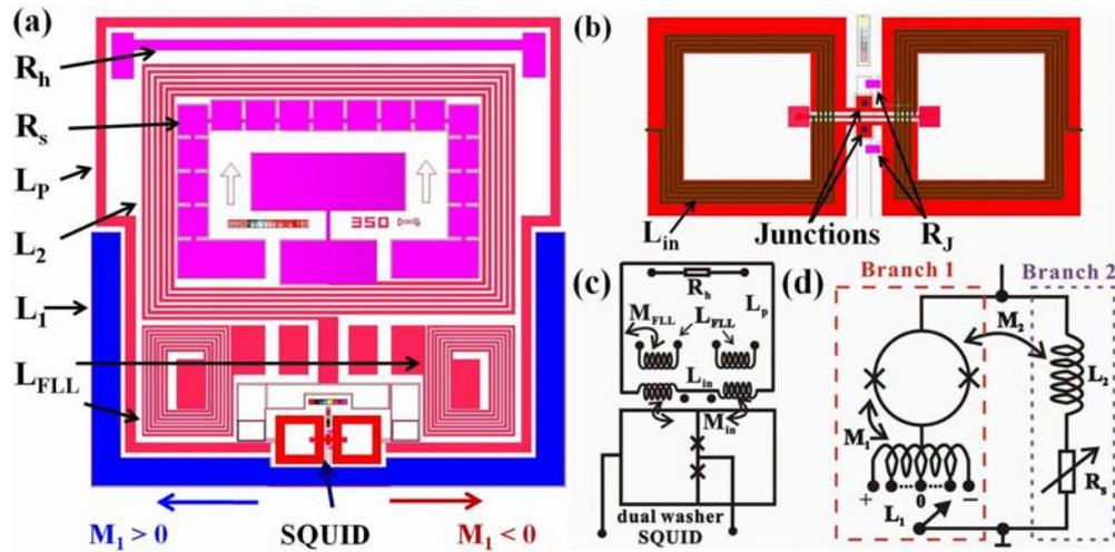
**Figure 1.** Layouts of (a) the SQUID chip with a size of  $5 \times 5 \text{ mm}^2$  and (b) the magnified dual-loop washer type SQUID with two opposite input coils with 4.5 turns each, also visible at the bottom of (a); (c) depicts the equivalent circuit of the SQUID magnetometer and (d) that of the bootstrap circuit [5].
