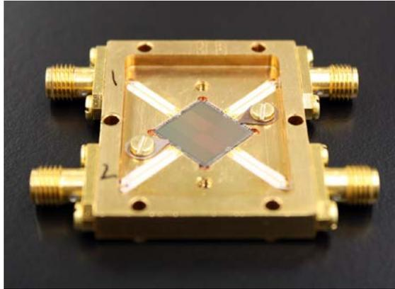
**Fig. 1.** (Reprinted with permission from Proceedings of the Astronomy Society of the Pacific). A 2024 pixel MKID array mounted in a microwave box.
