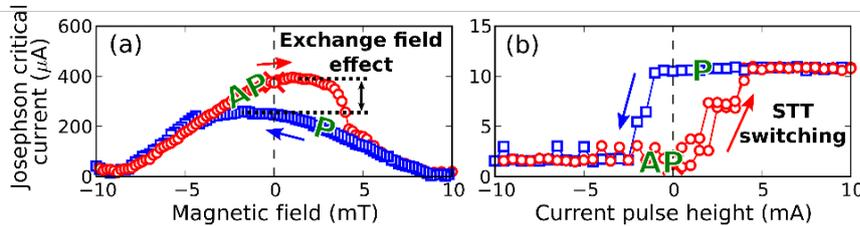
**Fig. 2.** Measured changes in maximum supercurrent. (a) Field switching in a micrometer-scale device. (b) Spin-transfer torque switching in a nanoscale device.
