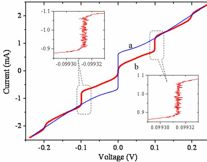
**Fig. 3.**  $IV$  characteristics of JJ array of 620 HTS junctions at 79.2K: (a) without and (b) with external mm wave irradiation at 77.465GHz. Enlarged portions demonstrate the amplitude and the steepness of the steps.
