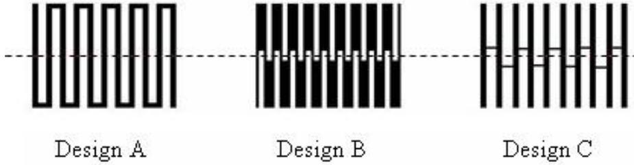
**Fig. 2.** Three different designs of Josephson junction arrays. The YBCO circuit is black, the GB is marked by the horizontal dotted line.
