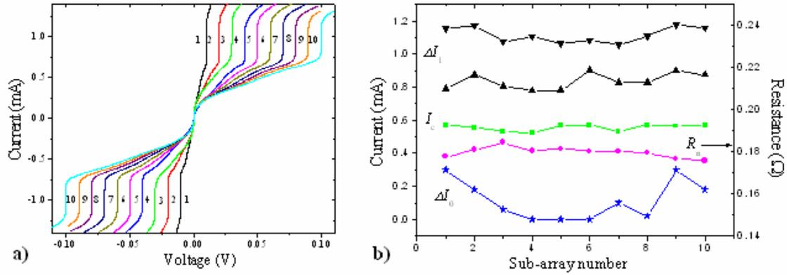
**Fig. 4** (a)  $I$ - $V$  characteristics of different HTS arrays at 79.2 K with external irradiation frequency  $f = 77.465$  GHz. The curves labelled from 1 to 10 denote the numbers of the sub-arrays of type B included in the arrays.
