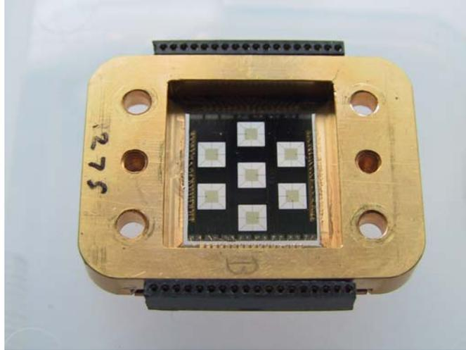
Fig. 4. Seven pixel detector array
