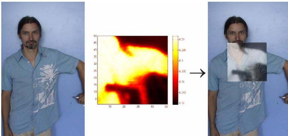
Fig. 10. Test scenario: a test person hides a handgun mock-up underneath his shirt, and the THz scan reveals the threat from 5 meter distance.
