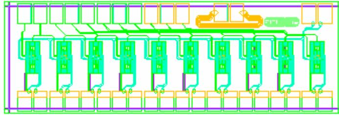
Fig. 5. Layout of the multiplexer
