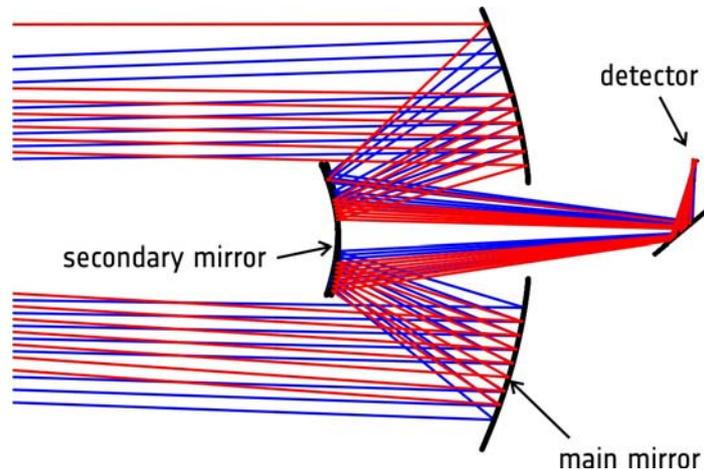
Fig. 1. Optical simulation with ZEMAX
