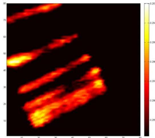
Fig. 7. THz image of a grating from Eccosorb stripes, recorded from 5 meter distance
