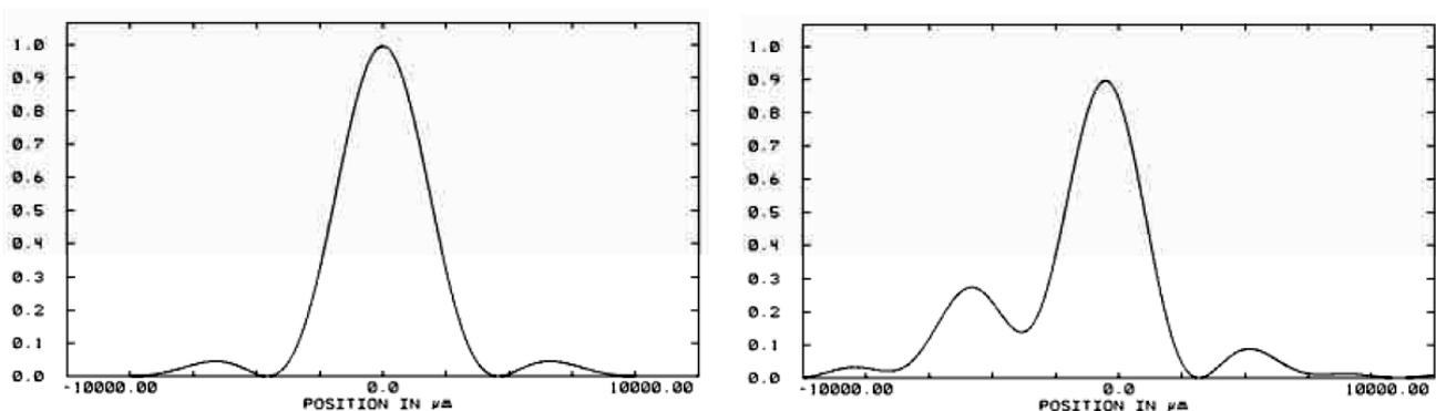
Fig. 2. Image of two point sources at  $4^\circ$  tilt of the secondary mirror
