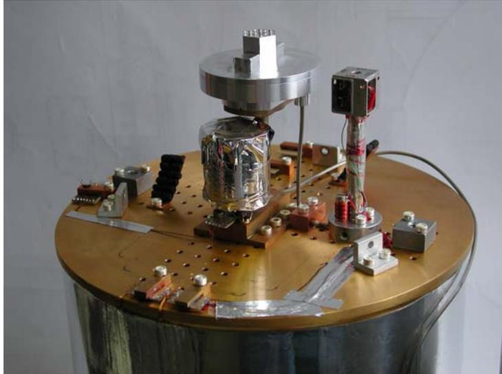
Fig. 6. Upside-down view on the cold plate of the cryostat, with the aluminium bolometer chamber atop.
