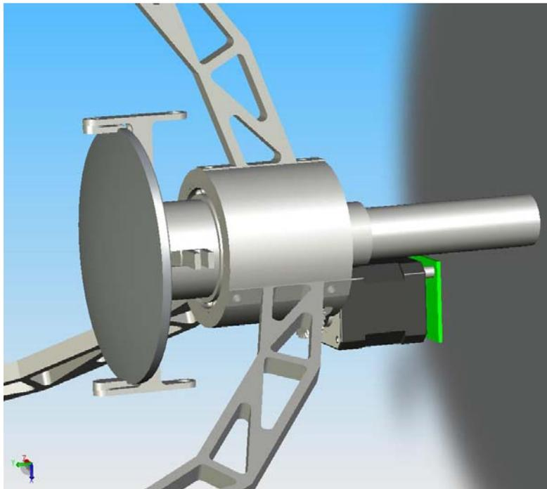
Fig. 3. Design of an optical scanner based on a gyrating mirror
