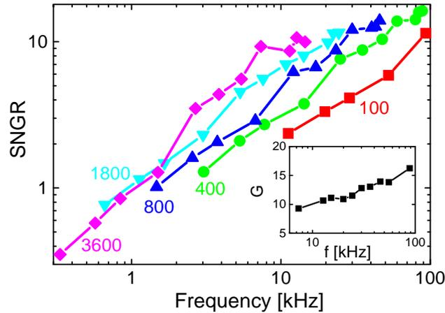
**Fig. 3.** SNR of LC circuits with coils of different windings and different shunt capacitors, measured at their respective resonance. The inset displays the maximum gain  $G$  obtained with the circuit working best at each frequency.
