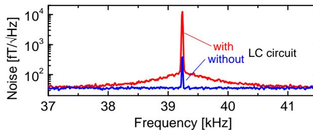
**Fig. 2.** Measured magnetic field noise density spectra without (blue) and with (red)  $LC$  circuit. Without the  $LC$  circuit, the signal and noise were  $384 \text{ fT}$  and  $35 \text{ fT}/\sqrt{\text{Hz}}$ , respectively; with the  $LC$  circuit, the signal and noise were  $12.3 \text{ pT}$  and  $108 \text{ fT}/\sqrt{\text{Hz}}$ , respectively.
