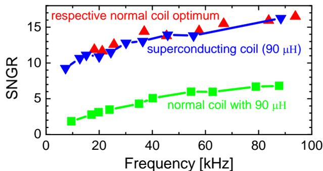
**Fig. 4.** Measured SNR of normal and superconducting coil circuits: blue – superconducting coil, red – maximum SNR of different normal coils at their respective optimum, green – normal coil with same inductance as superconducting coil.
