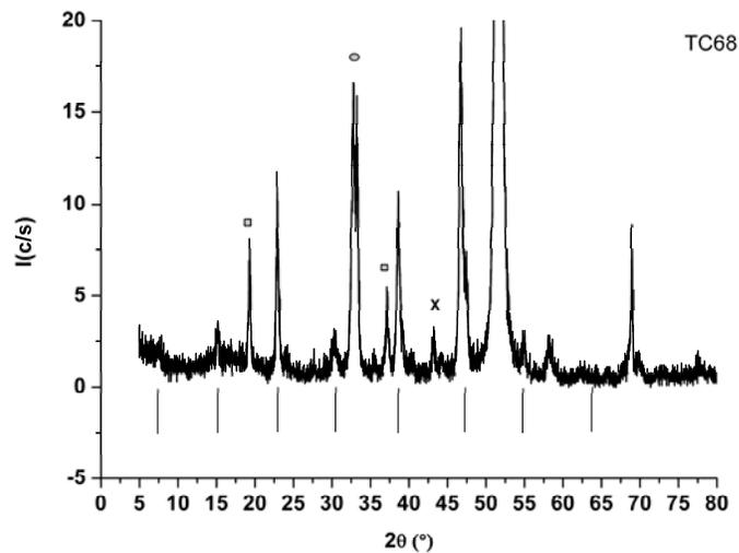
**Fig. 8.** X-ray scan of a healed tube covered with YBCO by MOCVD. Lines points to YBCO(001). Secondary phases are NiWO<sub>4</sub> (□), LZO (○) and NiO (x). The largest peak observed at  $2\theta = 51.61^\circ$  is due to Ni(200), suggesting a smaller W content than 5 at%.
