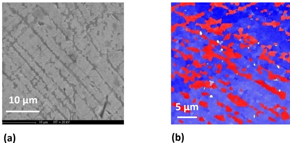
**Fig. 4.** Fractured LZO layer after the RW process. 4a: SEM of a RW tube where the initial tape was covered with LZO deposited by MOD process; 4b: EBSD of the same area, the red encoded areas correspond to Ni which crystal directions are rotated  $45^\circ$  from that of the LZO in blue.
