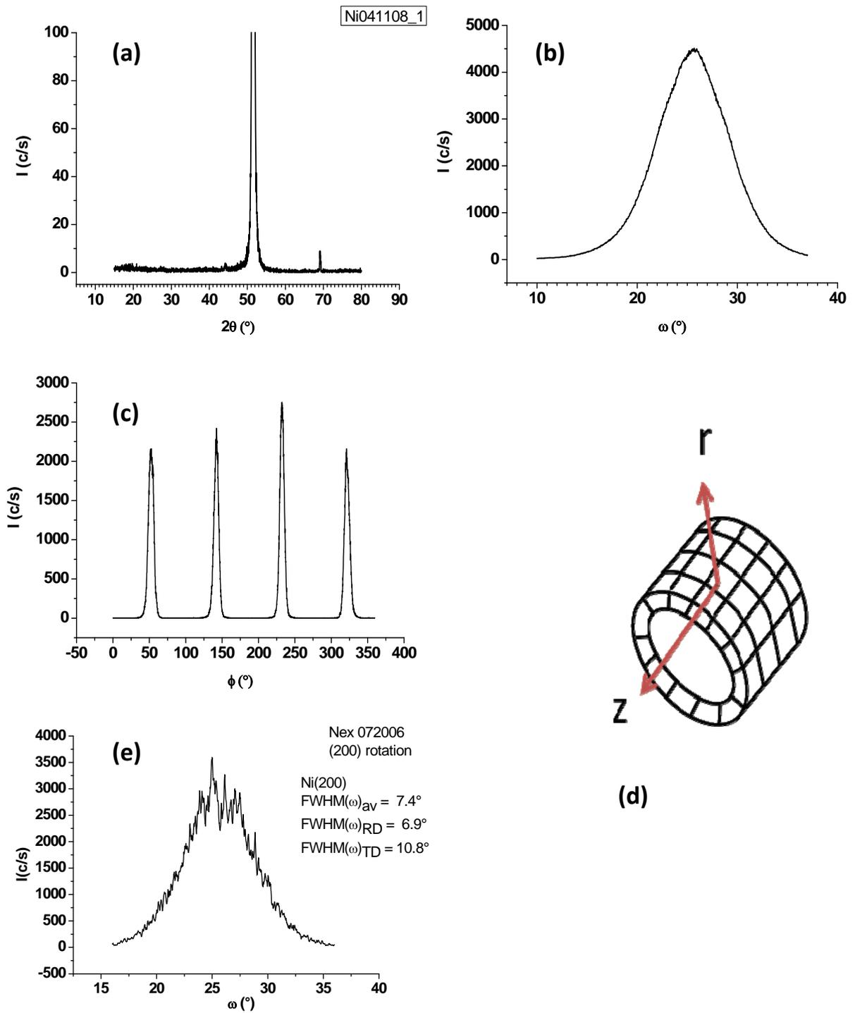
**Fig. 1.** Texture of a tube after the RW process: (a)  $\theta$ - $2\theta$  scan; (b)  $\omega$ -scan of (200); (c)  $\phi$  scan of (111); (d) schematic of the texture; (e)  $\omega$ -scan of the initial tape. The peak at  $69^\circ$  of Fig.1(a) originates from the substrate.
