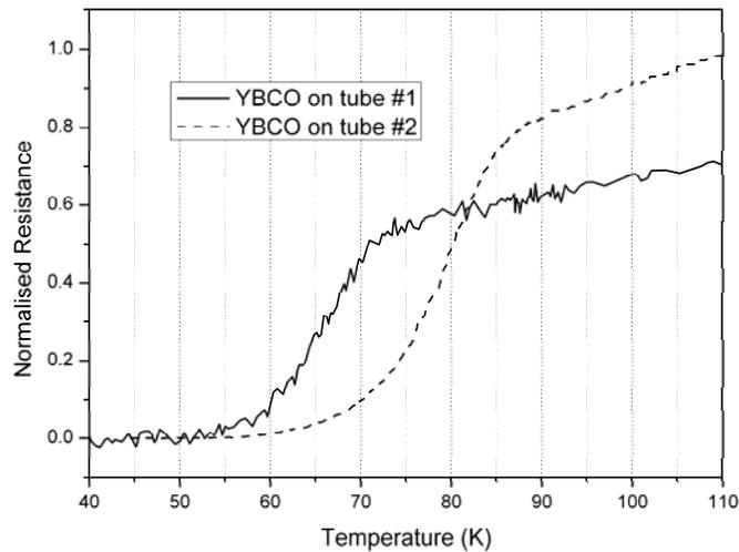
**Fig. 7.** Transport properties of YBCO textured tubes.
