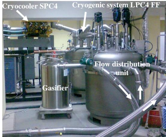
**Fig. 4.** Cryogenic system with flow distribution unit. Directions of LN<sub>2</sub> flows are shown.
