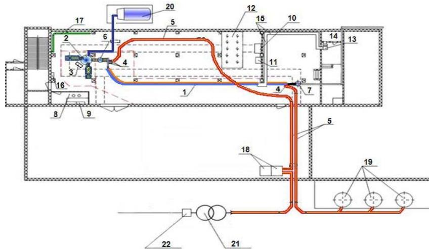
**Fig. 3.** Test facility for HTS power devices scheme. 1- HTS cable, 2, 3, 6, 7, 17, 20 – Cryogenic system, 4 – Current leads, 5, 11, 12, 16, 18, 21, 22 – Facility power system, 8, 9 – Facility control center 10 – DC current source, 13, 14, 15 – Air compartment, 19 – Electrical load.
