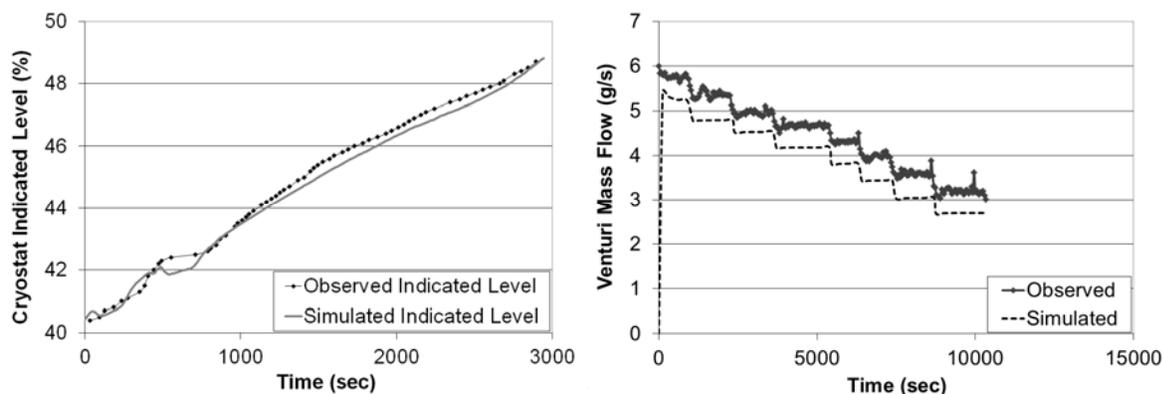
**FIGURE 3.** Simulated and actual results for cryostat filling (left) and cold gas return mass flows for various cryostat heater power settings (right). For the plot on the right heater settings are reduced in approximately 10 W steps over time from a high point of 70 W to a low point of 0 W, and the flows are measured using a venturi located on the cold gas return line about 3 m from the cryostat.
