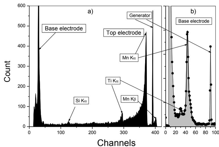
Fig. 1. Pulse height spectrum of the STJ detector Ti/Nb/Al<sub>x</sub>/Al/Nb/NbN at  $V_d = 0.59$  mV: (a) total spectrum and (b) subspectrum of the bottom electrode. Layer thicknesses are 30/150/4,2/13/250/30 nm; the detector area is  $6400 \mu\text{m}^2$ .
