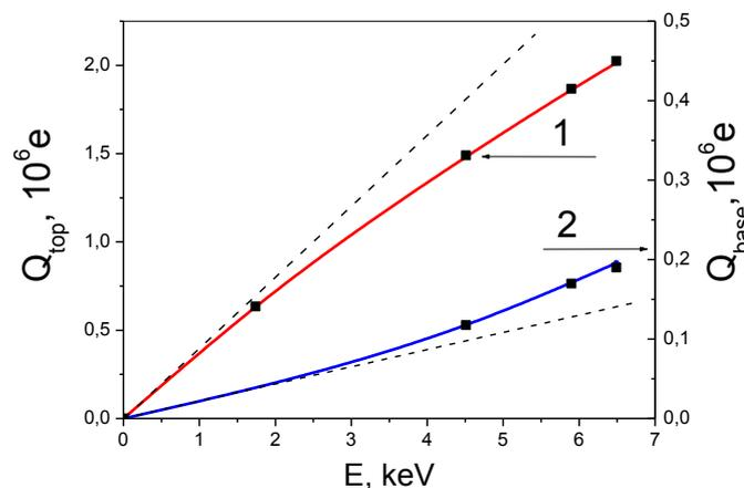
**Fig. 2.** Dependences of the signal amplitude on the X-ray energy for the top electrode (1) and the bottom electrode (2);  $V_d = 0.59 \text{ mV}$ . Squares are the experimental data. Solid lines are the diffusion model calculations. Dash lines show the linear response.
