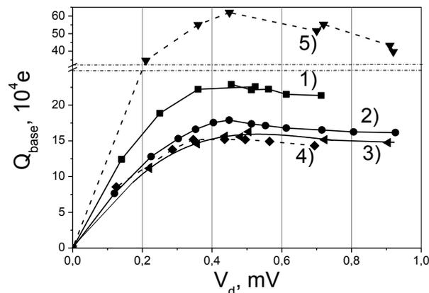
**Fig. 3.** Signal amplitudes of Nb–Ti (1–4) and Nb–Al (5) killed electrodes in STJ detectors as functions of the voltage  $V_d$  for samples with electrode thicknesses  $d_{\text{base}}$ ,  $d_{\text{top}}$ , and  $d_{\text{Al}(2)}$ : (1) 130, 193, and 13 nm; (2) 180, 243, and 13 nm; (3) 180, 293, and 13 nm; (4) 180, 243, and 12; (5) 90, 145, and 15 nm.
