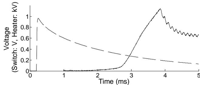
**Fig. 7:** Voltage across a switch utilizing YBCO-SS (solid line) and across the heater (dashed line). The induced voltages in the laminations and substrate of the YBCO-SS by the heater pulse have been removed. After 4 ms the voltage of the switch current source reached the predetermined threshold and so the current was automatically decreased in order to protect the HTS.
