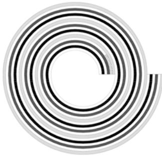
**Fig. 6.** Schematic of a switch (not to scale) showing the non-inductive bifilar HTS winding co-wound with a resistive heater and insulation. The current and voltage terminals, support, and outer insulation/heater section have been omitted for clarity. White regions represent insulation, black the heater, and light and dark grey the HTS which were soldered together over the crossed region.
