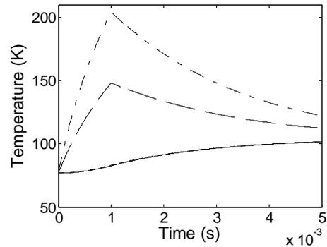
**Fig. 4.** Temperature profiles at the mid point of the heater (dash-dot line), the insulation between heater and HTS (dashed line), the YBCO-Cu (solid line). The temperature of the insulation between HTS layers is virtually identical to that of the YBCO-Cu layer.
