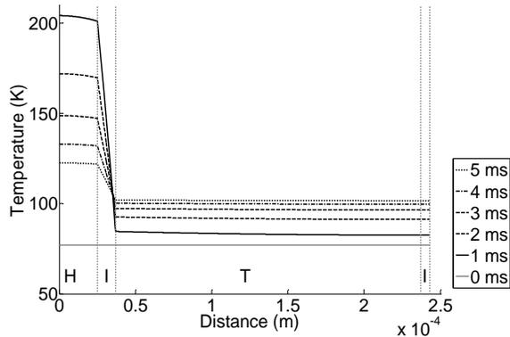
**Fig. 3.** Temperature at 0.5 ms intervals through the switch. Dashed lines represent temperature whilst the heater is on, dotted lines when it is off. The solid line is at the instant the heater turns off. The vertical lines bound regions of the switch with H representing the heater, I insulation, and T YBCO-Cu tape.
