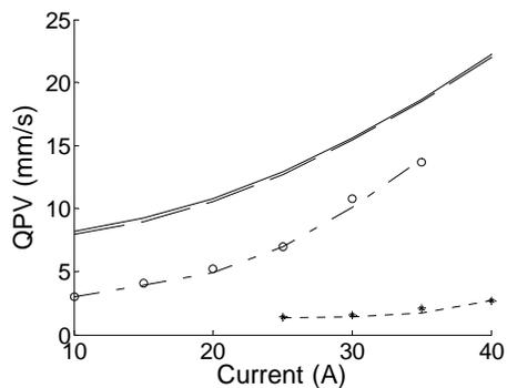
**Fig. 2.** Calculated and measured QPVs for YBCO-SS with different transport currents and cooling. The solid line represents the PDE model with no cooling and a 3.6 W heater, dashed line 3.2 W; dash dot line with low cooling and lower heater power, dotted line with high cooling and higher heater power. Circles represent measured data for YBCO-SS with low cooling and a 3.2 W heater; stars represent measured data for YBCO-SS with high cooling and a 3.6 W heater.
