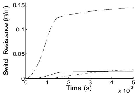
**Fig. 5.** Comparison of modelled switch resistances as a function of time. The solid line represents a switch made of YBCO-Cu, dashed line a switch of YBCO-SS, dotted line a switch of BSCCO-Ag/Au.
