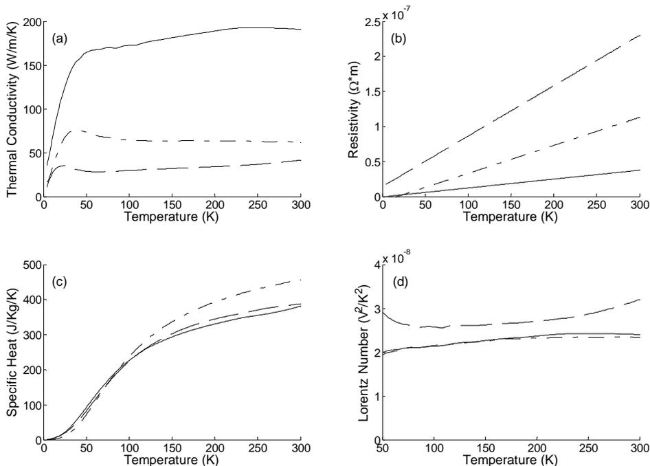
**Fig. 1.** (a), (b), & (c) show measured thermophysical properties; (d) shows calculated Lorentz numbers. Solid lines represent YBCO-Cu, dashed lines YBCO-SS, and dash-dot lines  $MgB_2$ -Ni/Cu/Fe.
