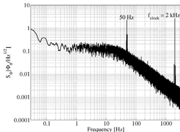
**Fig 2.** Measured flux noise spectral density of the digital SQUID magnetometer in unshielded conditions. No external field is applied (only the Earth's magnetic field is present). The clock frequency is 2 kHz. The duration of measurements is 128 seconds.
