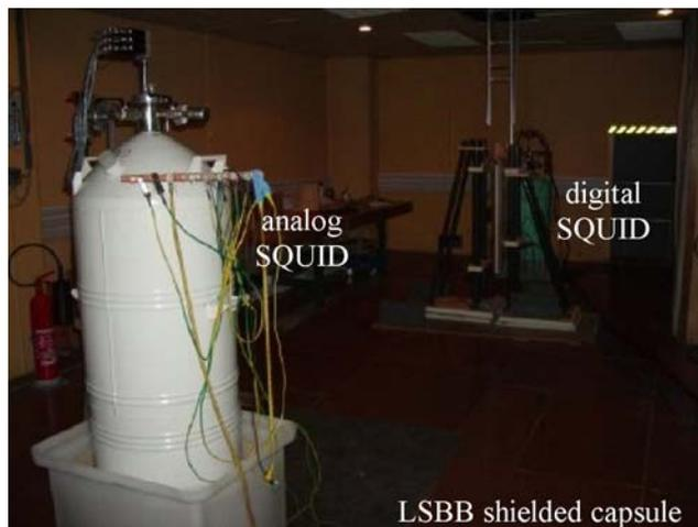
**Fig 3.** Setup of analog and digital SQUIDs in the shielded capsule at the low-noise facility of LSBB in Rustrel.
