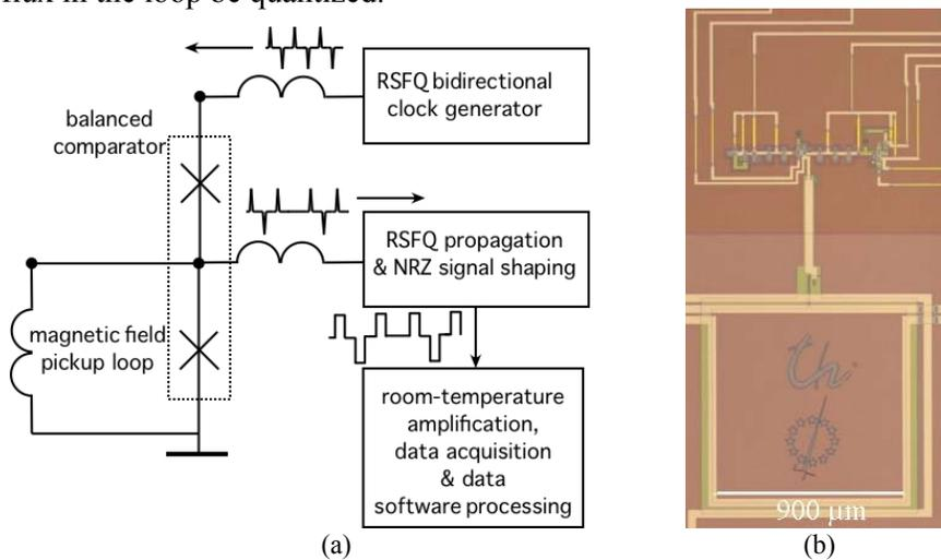
**Fig 1.** (a) Block diagram of the digital SQUID magnetometer. The balanced comparator is composed of two identical Josephson junctions; (b) photo of the device (courtesy of IPHT Jena): the pickup loop is seen at the bottom while the top central part connected to the loop is the balanced comparator. The top left part is the clock generator while the signal propagation and pulse shaping circuit is located to the right of the comparator.
