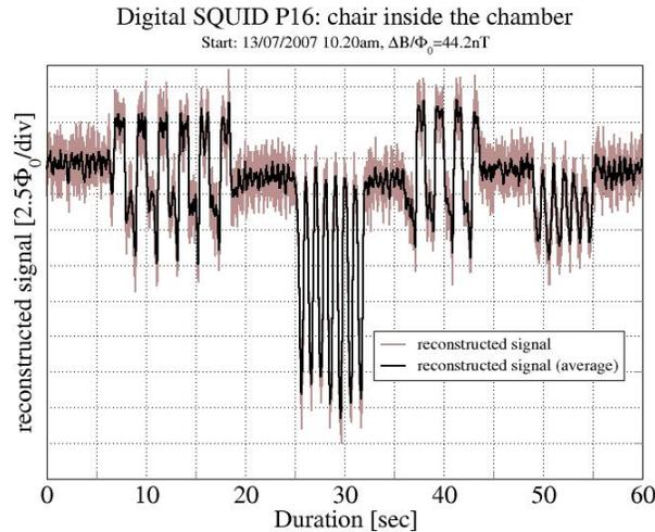
**Fig 4.** Reconstructed signal after post-processing of the digital SQUID data obtained in presence of a magnetic perturbation artificially created in the shielded room. The red curve corresponds to the measured signal while the black curve is obtained by doing a running average of the red curve to cancel most of the unwanted noise. The digital SQUID device used for these measurements had a sensitivity about 10 times lower than the optimized one, whose noise spectrum is given in Figure 2.
